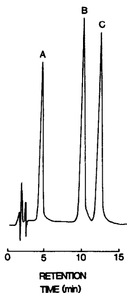
Fig. 1. HPLC of penicillin X (30 \mu\text{g/ml} ) (A), penicillin G (30 \mu\text{g/ml} ) (B) and penicillin V (40 \mu\text{g/ml} ) (C), following pre-column derivatization with an imidazole-mercury(II) chloride reagent. Flow-rate = 1.5 ml/min; injection volume = 20 \mu\text{l} ; detector sensitivity = 0.2 a.u.f.s.; detection wavelength = 325 nm. Mobile and stationary phases are given in the Experimental section.
